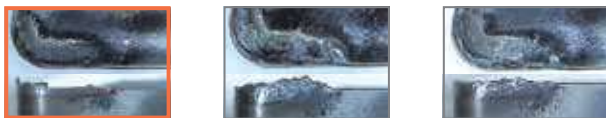
Work Material: GG-25, Continuous, Insert: CNMG120408 Cutting Conditions: v_c = 600 m/min, f = 0,4 mm/rev, a_p = 2,0 mm, dry
