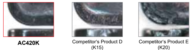
Work Material: GGG-40.3, Toolholder: PCLNR2525-43 Insert: CNMG120408 Cutting Conditions: v_c = 350 m/min, f = 0,25 mm/rev, a_p = 1,5 mm, wet
