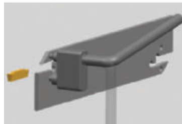
② Clamp the insert on its seat after turning the handle to 45°~160° for loosening the seat.
